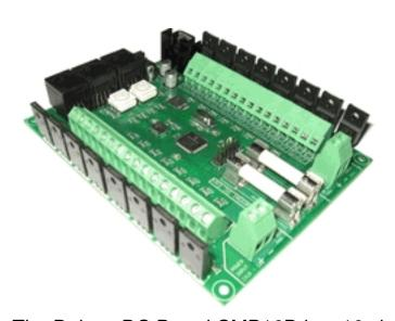
The Deluxe DC Board CMB16D is a 16 channel controller that can operate independently.
